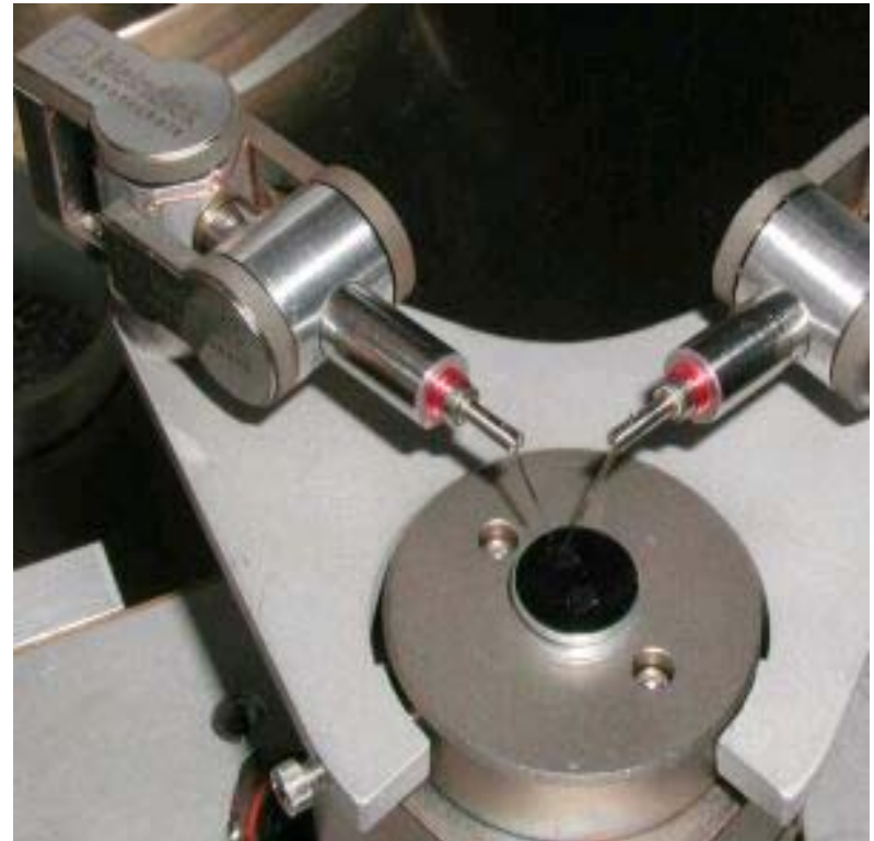
Precision positioning and picking up of individual particles by means of microtips (down to 100 nm)
