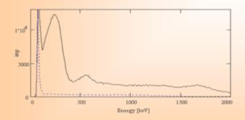
Sample of Fe-ore, HPGe detector, counting time T=144000 s
