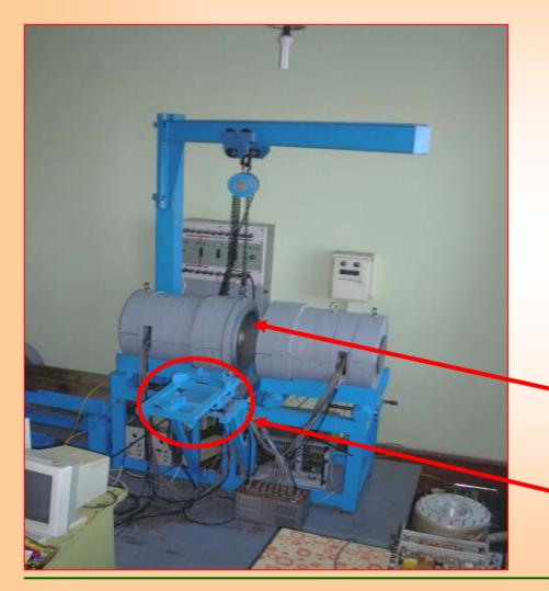
For high resolution, low-gamma active measurements is possible to be applied Anti Compton and Anti Background approach, as  $4\pi$ -multidetector system Romashka is set as an active shielding of Ge detector
