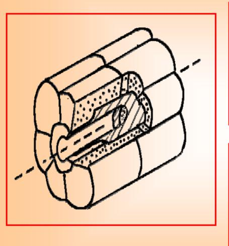
$4\pi$  - multidetector system ROMASHKA (Daisy) for gamma low activity measurements is assembled from 12 scintillators NaI(Tl) which are divided on two halves of 6 crystals with a special shape (like a flower Daisy). The crystals measure in total are 16.6 l NaI(Tl) and they are placed in a cylinder with the outside diameter 30 cm
