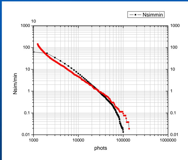
The simulation shows that the energy threshold of the detector is about  $5 \cdot 10^{13}$  eV
