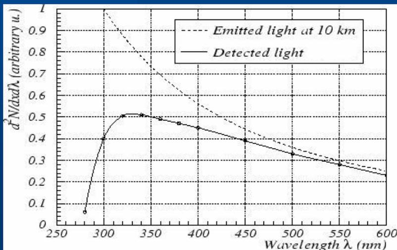
*Differential Cherenkov photon spectrum. Continuous line includes absorption by ozone and Rayleigh and Mie scattering. The spectrum has a peak at around 350 nm.*
