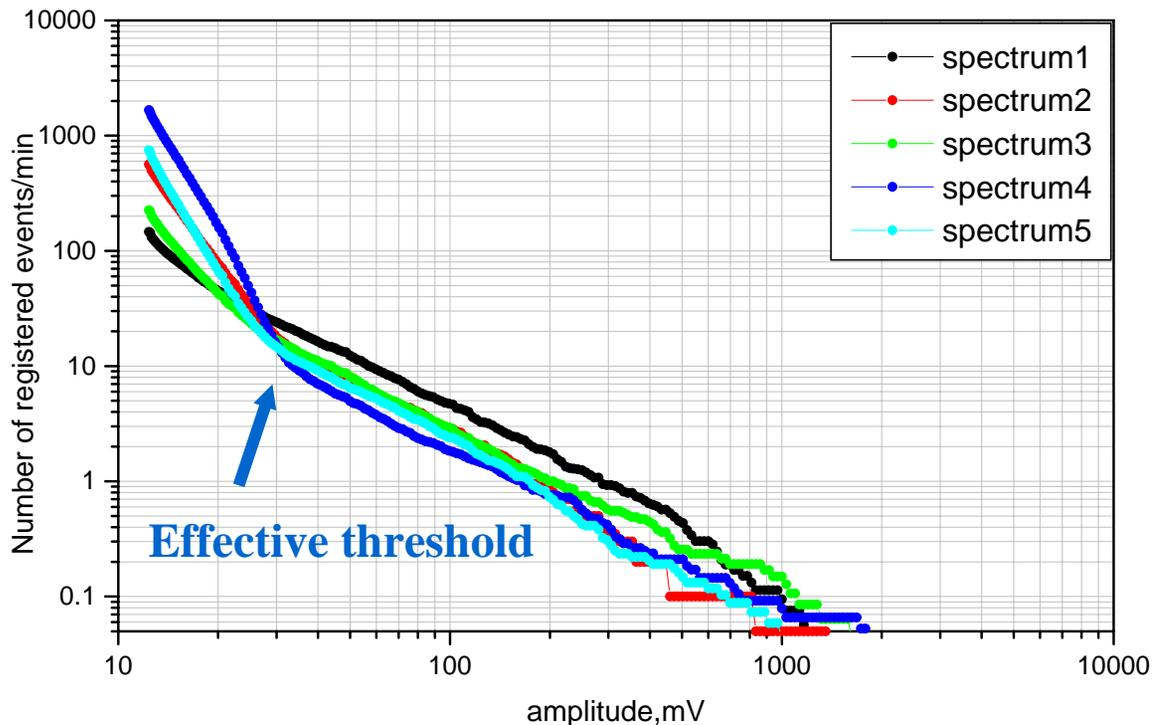
The *spectrum1* (black line) was obtained with simultaneous operation of RMR LIDAR, i.e. in very good atmospheric conditions. The next were obtained during changeable atmospheric conditions above the telescope.
